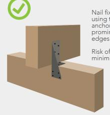
Nail fixing roof trusses using triple grip framing anchors reduces the prominence of exposed edges.
