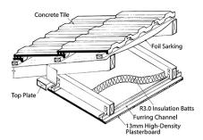
Concrete tile roofing, with foil sarking under battens. 13mm thick dense plasterboard on steel furring channels. Rw = 52 Rw + Ctr = 46 Consistently, test figures show equal, or slightly improved roof noise attenuation performance for tiles compared to sheet steel for the Weighted Sound Index (Rw) and a significant improvement (9% to 12%) for tiles compared to sheet steel for the Weighted Sound Index with Spectrum Adaption (Rw + Ctr).
